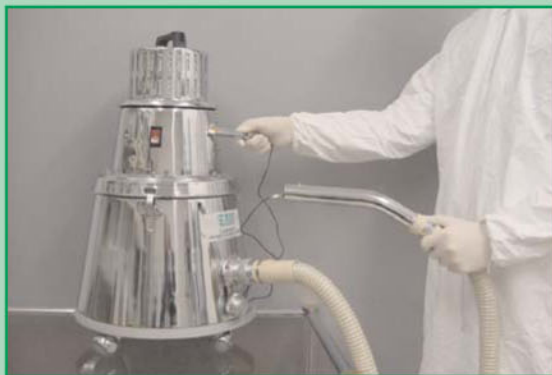
Fig. 1 Ground tester to verify continuity
